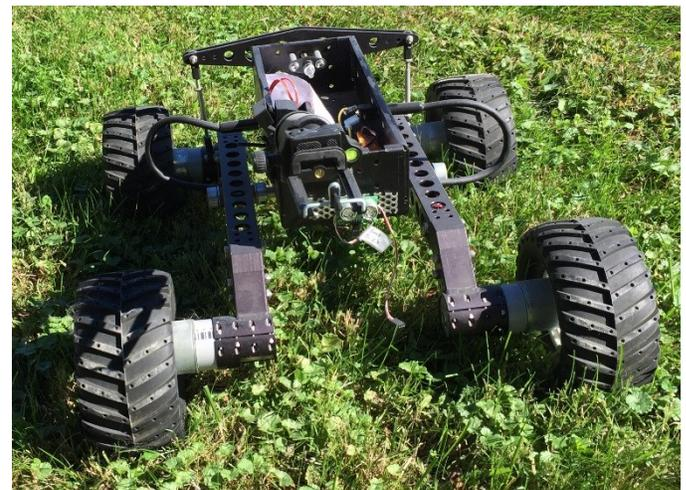
Figure 3: Robotic Rover Used to Capture Video for Testing
